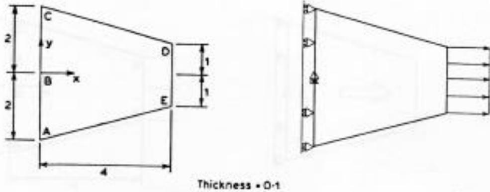
LOADING                      Uniformly distributed horizontal load of 10MN/m (pressure of 100MPa) along outer edge DE
