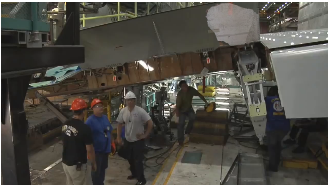
Figure 8: Inboard Spoilers, B777 Production Line (recovered article as overlay)
