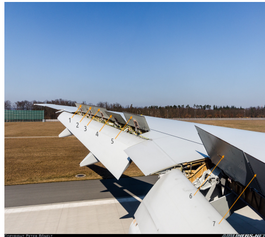
Figure 6: B777 Spoilers Deployed, Left Wing
